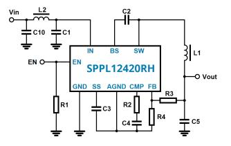
For given values of the R4 resistor and the  $V_{_{FB}}$  chip reference voltage, the R3 resistor may easily be calculated for the desired output voltage.
