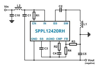
With monolithic POL converters very simple and efficient circuits cover operation of a huge diversity of payload modules with different supply voltage requirements from a standard intermediate voltage. The minimum of passive external components ensures a very cost- and space-saving design.
