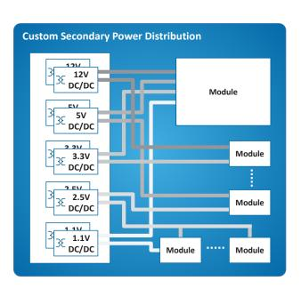
efforts. Any alterations in the payload architecture necessarily entail changes in the design of the power supply unit. At the same time, the power distribution to the modules with low voltages and high currents requires heavy power rails due to large cross-sections or suffers from conduction losses or both.
