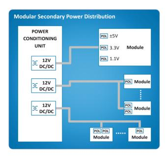
The evolution of power distribution in spacecraft goes into direction of modular architecture. Especially secondary power distribution from the satellite bus to the modules can be made more efficient by applying modular design.
